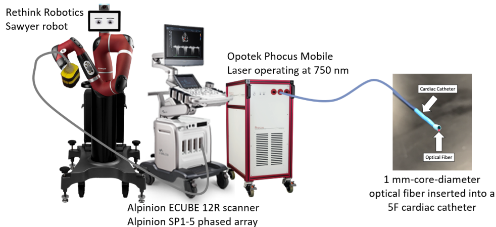
Figure 2: Robotic-photoacoustic imaging system equipment. The Alpinion SP1-5 phased array was held by the end effector of the robot with a custom 3D printed holder. A 1 mm-core-diameter optical fiber was coupled to the output port of the laser on one end with its other end inserted into, and coincident with the tip of, a 5F inner diameter (7F outer diameter) cardiac catheter to create a fiber-catheter pair.
