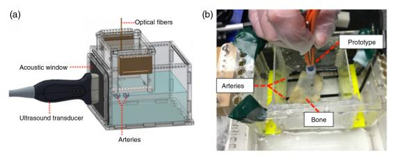
Fig. 5 (a) Solid model of phantom and (b) experimental setup with light delivery prototype used to image through a cadaveric bone specimen.
