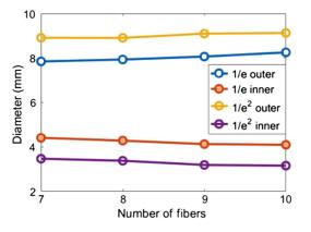
**Fig. 10** Inner and outer diameters of 1/e and  $1/e^2$  beam profiles detected on a planar surface that is coincident with the drill tip and orthogonal to the drill axis.
