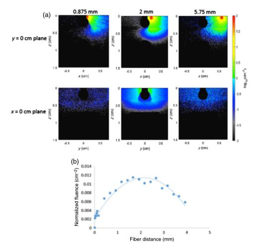
**Fig. 6** The distance of the fiber from the drill shaft alters the normalized fluence distribution. The images (a) display the normalized fluence when the fiber is located at distances of 0.875, 2, and 5.75 mm from the drill shaft (as indicated above each image), while the plot (b) shows measured data points along the artery surface as a function of multiple fiber distances. The quadratic curve  $F_N = -0.002d_f^2 + 0.0086d_f + 0.0021$  was fit to the data points.
