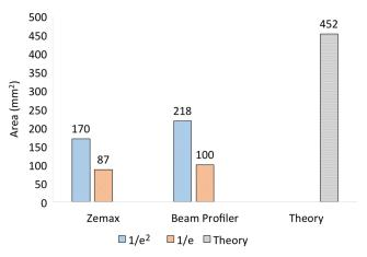
**Fig. 14** Measured 1/e and  $1/e^2$  spot sizes at a distance of 20.1 mm away from the fiber surface. The theoretical approximation for the total beam size is shown for reference.
