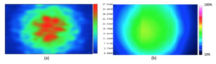
**Fig. 13** Beam profile 20.1 mm away from the fiber surface measured with (a) Zemax and (b) the beam profiler. The peak intensity is lower than 100% with the beam profiler result because data are not normalized. The dimensions of these images are 11.3 mm  $\times$  18 mm.
