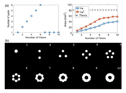
**Fig. 9** (a) Number of spot sizes observed and 1/e area of the spot sizes as a function of the number of fibers surrounding the drill. (b) Images showing the 1/e thresholding used to calculate area as the number of fibers increased. The beam profiles converge with seven or more fibers.
