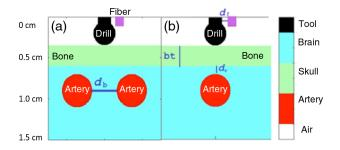
**Fig. 3** Monte Carlo Simulation diagram. (a) Two vessel simulation. The variable in this simulation was the distance between two arteries  $(d_b)$ . (b) Single vessel simulation. The variables in this simulation were bone thickness (bt), distance between artery and bone  $(d_v)$ , and distance between the fiber and the drill shaft  $(d_f)$ .
