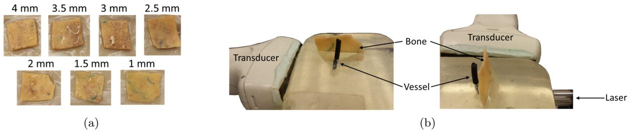
Figure 1. Photographs of (a) skull bone sanded to the thicknesses indicated above each image and (b) the experimental setup.
