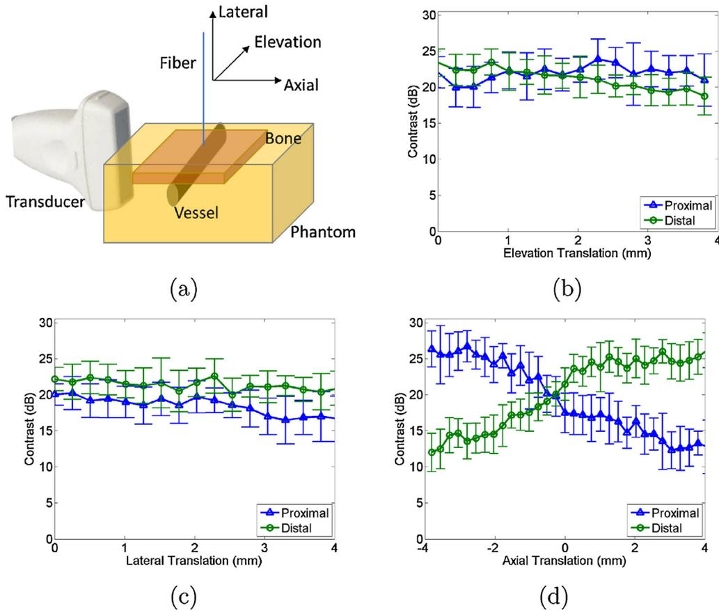
**Fig. 7.** (a) Schematic diagram of phantom and experimental setup. Mean contrast as a function of fiber translation in the (b) elevation, (c) lateral, and (d) axial probe dimensions. Error bars represent  $\pm$  one standard deviation of twenty measurements. Schematic diagram illustrates fiber translation directions.
