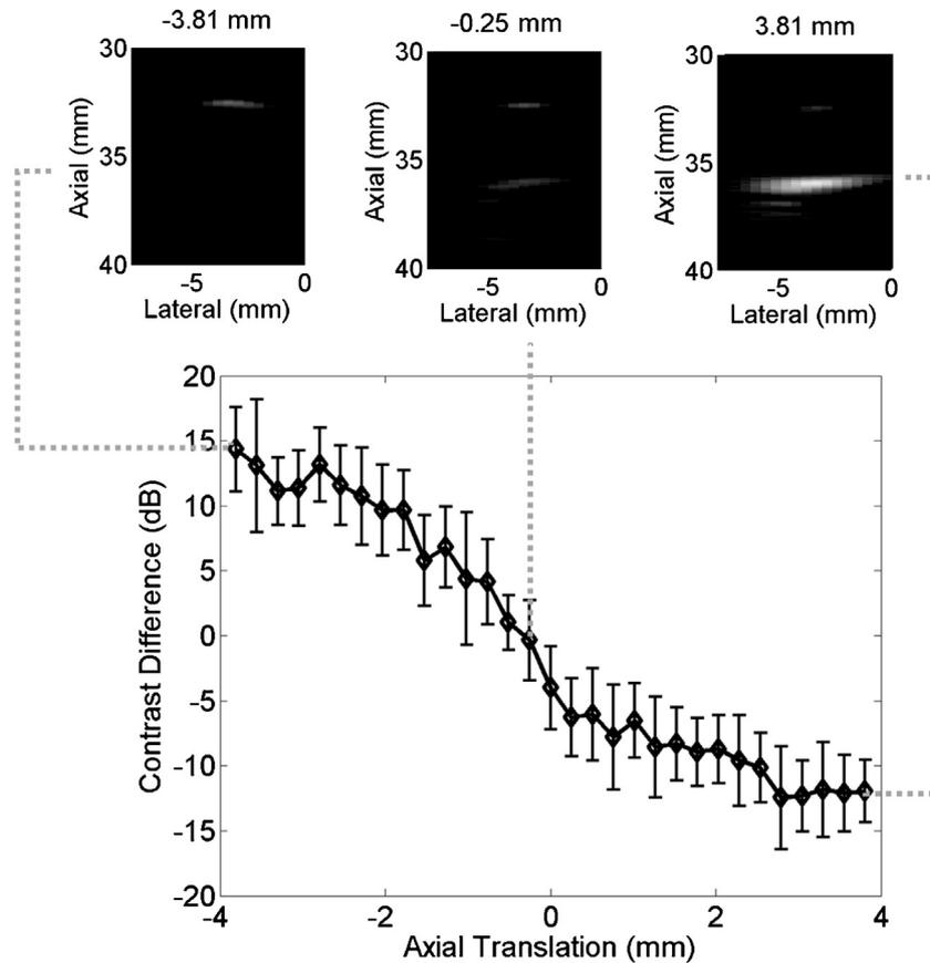
**Fig. 8.** Mean contrast difference between the proximal and distal vessel boundaries as a function of fiber translation in the axial probe dimension. Error bars represent  $\pm$  one standard deviation of twenty measurements. The example photoacoustic images show vessel boundaries visualized at fiber positions -3.81, -0.25, and 3.81 mm, from left to right, respectively. All images are shown with 20 dB dynamic range.
